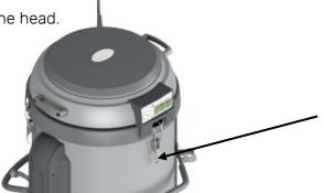
> Lift the motor head and rest this on a support bench.
