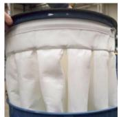
Loosen the clamp and remove the support ring with seal
