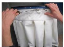
Remove the knots and take out the pocket filter. Fit the new filter and put everything back in place, locking the cap.
