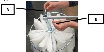
> Remove the filter with its complete support
