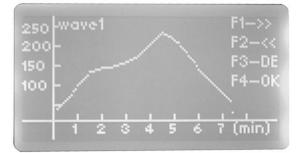
② Following we provide eight different waves, please choose one according to your request. Press the F1/F2 to choose different wave, press F3 to look into different wave parameter, press 4 to confirm the wave you chose.
