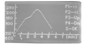
Press "F1/F2" button, forward and backward to select different time. Press F3/F4 button up and down to select different temperature, Press "s" button to save.
