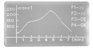
Press "F3" button again to see the parameters for the chosen wave, for example soldering paste sort, soldering temperature, time etc.
