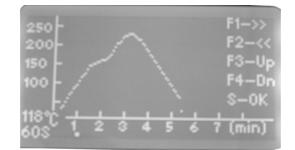
Press the "F1/F2" buttons forward and backward to select different times. Press "F3/F4" buttons up and down to select different temperatures, press "S" button to save.
