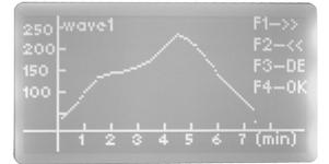
Press the "F3" button again to see the parameters for the chosen wave, for example soldering paste sort, soldering temperature, time etc.
