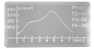
② Following we provide eight different wave cycles, please choose one according to your request. Press the F1/F2 to choose a different wave, press F3 to look into different wave parameters, press 4 to confirm the wave you chose.
